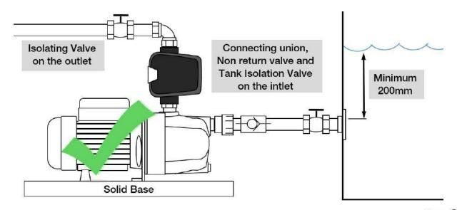
In this example the water level is higher than the pump inlet but the water cannot flow freely into the pump.
