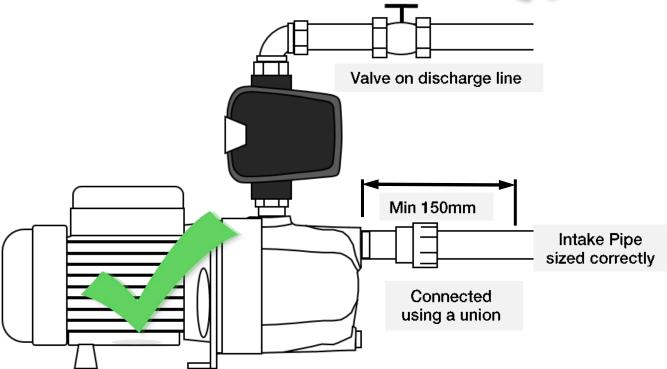
Optional: If the water is known to contain particles (sand etc.) an in-line strainer/filter can be fitted. Usually 500 micron is sufficient, Regular maintenance is required to keep an in-line strainer/filter clean and ensure best pump performance.
